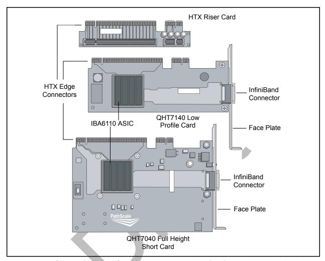
Figure 4-3. QLogic QHT7040/QHT7140 Full and Low Profile Cards with Riser, Top View
